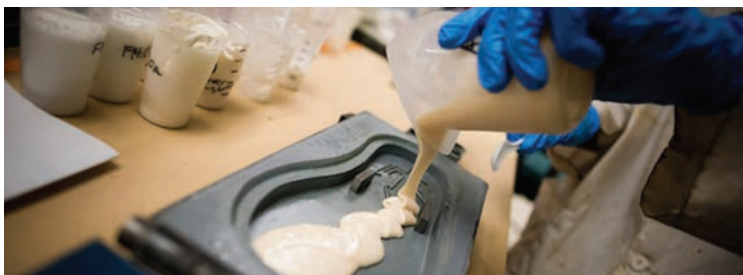
Pouring algae-derived polyol into flip-flop mold (Photo by Erik Jepsen/UC San Diego)
